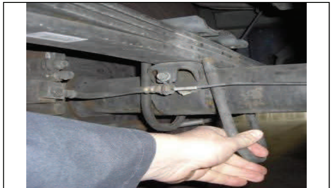
Remove u-bolts and carefully lower axle.
