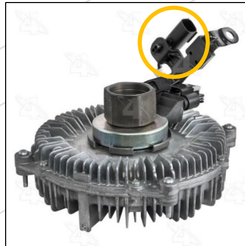
Figure 16: Cooling Fan Electrical Connector
