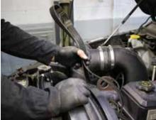
Remove factory idler pulley and replace with supplied smaller pulley utilizing the factory bolt, spacer, and supplied washer. Install back onto the engine.
