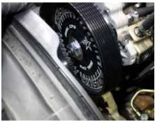
Install supplied serpentine belt. Follow the diagram below to route correctly.
