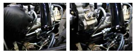
Install fuel supply and fuel return lines from the brass T's previously installed into the factory fuel lines to the secondary pump, use supplied clamps and tighten.
