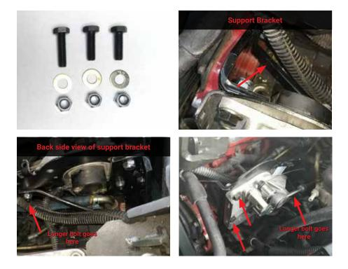
Install supplied 45° radiator hose connection onto the thermostat housing, then install supplied upper radiator hose re-location pipe as shown using factory bolt.
