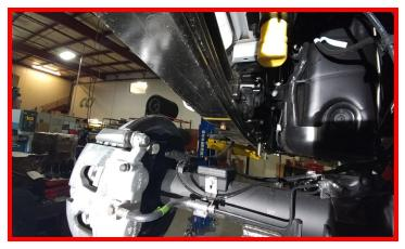
Locate the driver side lift block (Has a D cut into it under the bump stop tang). Raise the axle and the block up to the spring while aligning the center pin. Install the provided u-bolts, and nuts. Snug the u -bolt nuts but **do not fully tighten at this time**. Repeat steps for passenger side.
