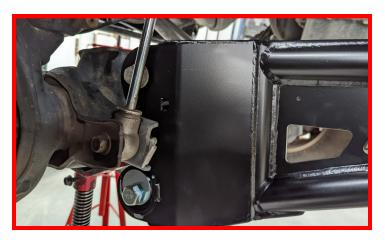
Rotate the axle until you can line up the ReadyLIFT radius arms with the factory hole. Install using factory hardware.
