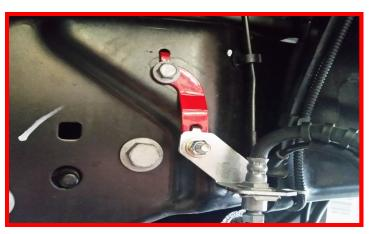
Reattach the factory brake line bracket at the axle using factory hardware.
