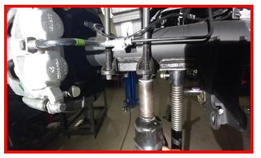
Lower the axle just enough to remove the factory block, making sure not to over extend brake and ABS lines. Adjust as necessary.
