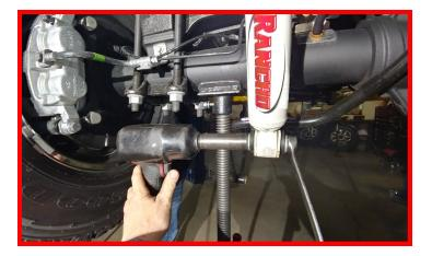
Slightly loosen but do not remove the passenger side u-bolts. Remove the driver side u-bolts completely.
