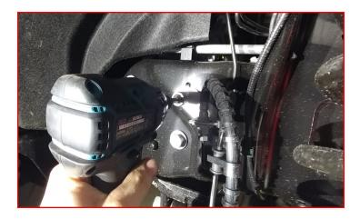
Remove the brake line bracket at the axle.
