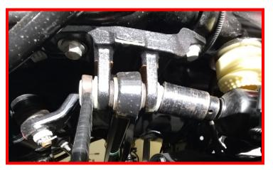
Remove factory track bar bracket and discard. Using the factory hardware, install the supplied track bar bracket on the frame in the factory orientation.
