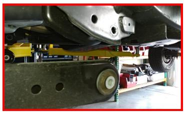
Remove vacuum line from driver side factory radius arm.
