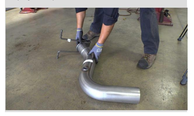
7. Install a 5" exhaust clamp onto the inlet of the Rear Tailpipe & Install the Rear Tailpipe onto the outlet of the Front Tailpipe.
