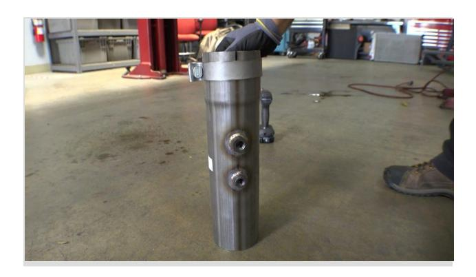
6. Slide a 4" exhaust clamp onto the front of the Banks front tailpipe.
