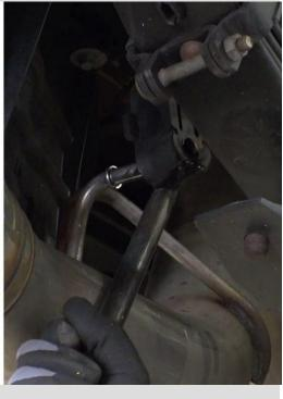
NOTE: Lubricating the rubber hangers with WD-40 or similar lubricant will ease the removal of the hanger pins.
