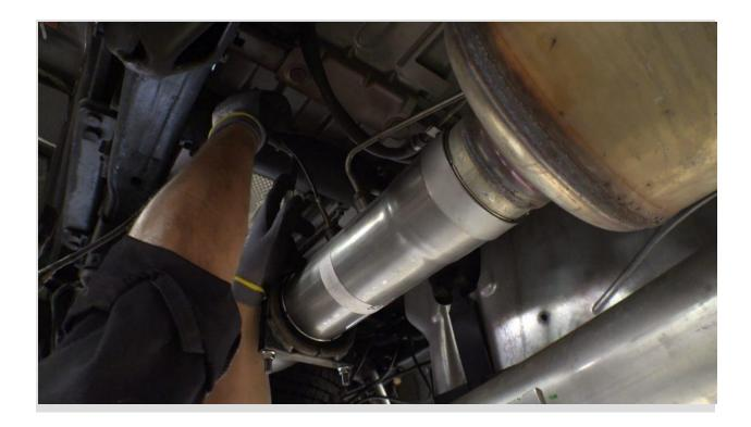
8. Engage the factory rubber hangers onto the hanger clamp pins.
