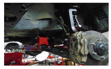
Install the OEM brake line bracket to the ReadyLift steering knuckle using factory hardware torque to 10 ft-lbs.
