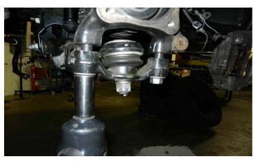
Remove lower strut hardware. Loosen the lower control arm (LCA) cams and let the LCA swing out of the way.
