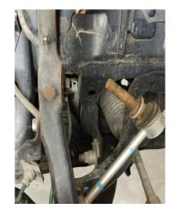
Loosen but do not remove the upper ball joint nut. Strike the ball joint boss with a hammer to dislodge the taper.
