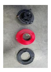
Release the spring tension and remove the factory top hat. Add the ReadyLIFT Spring spacer align the three relief pockets in the spacer to the studs on the top hat. Use the rubber isolator between the spring and aluminum spacer. Realign the alignment marks and compress the strut assembly. Reinstall the containment nut and torque to 35 ft-lbs.
