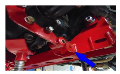
Lower the axle and differential down to the passenger side bracket start the original factory bolts, do not tighten. Rotate the driver side bracket to the differential add the three laser cut washers between the bracket and the differential use the original factory bolts to fasten. Do not tighten at this time.
