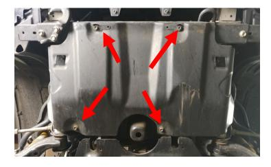
Remove the differential gravel guard.
