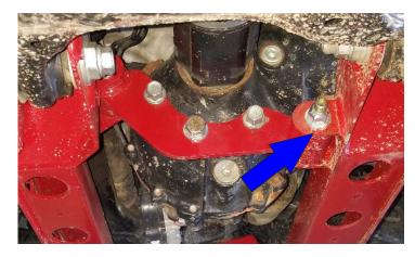
Reinstall the lower control arm to the ReadyLift crossmember use the original factory hardware. Do not tighten at this time.
