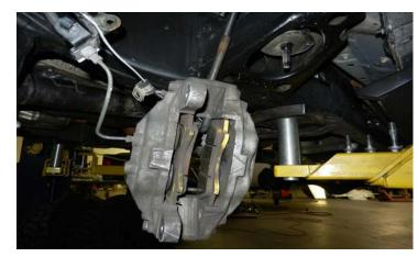
Remove the safety clip from the upper ball joint, cotter pin from the tie rod ends, and axle nut.
