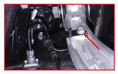
Remove the ABS sensor harness and brake line bracket from the knuckle and hang out of the way. Retain the factory hardware.
