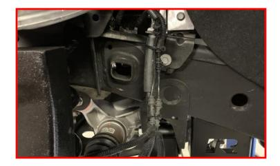
Install the sway bar drop link into the lower control arm using factory nut.
