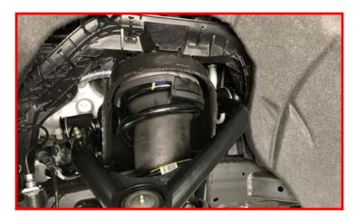
Note the installation orientation. The mounting bolts are facing toward the front of the vehicle and extension offset toward the center of the vehicle.
