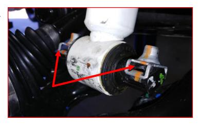
Locate the front clamshell strut extensions and hardware. (M12 x 25mm bolts, washers, M10 x 40mm bolts, M10 x 50mm bolts, washers and locking nuts) You will see the lower strut extensions are labeled with a "D" and "P". This is to identify the location the extension is to be installed. "D" corresponds with the driver and "P" corresponds with the passenger side. This orientation is important to prevent damage to other suspension and driveline components. Passenger side shown.
