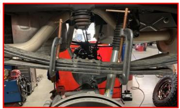
Remove the center pin holding the leaf pack together. Discard center pin.
