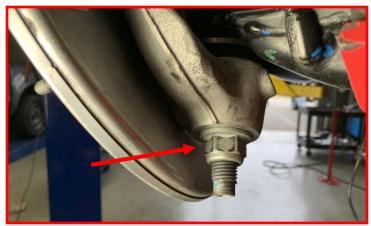
Remove upper control arm bolts located inside strut tower. Retain the factory pivot hardware. Discard factory upper control arm.
