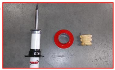
Install the billet pre-load spacer on top of factory spring perch. The spacer should nest onto the factory spring perch.
