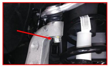
Support the lower control arm with a suitable jack. Remove the lower strut mounting bolts from the lower control arm. Discard factory bolts.
