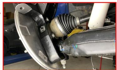
Note: driver side CV axle will receive a 1/4" aluminum spacer. Install the spacer onto the CV axle with the chamfered side towards the axle.
