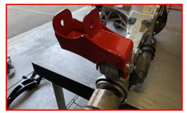
Install driver side differential drop on factory differential mounting point using the supplied M14 x 90mm bolt, washers and nut. Do not tighten at this time.
