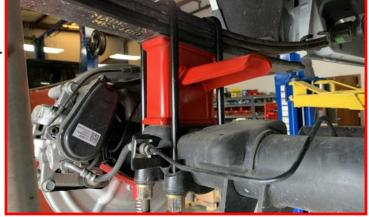
Install the performance aftermarket shock into the frame using factory hardware. Do not tighten at this time.
