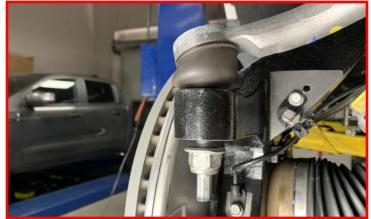
With everything tightened and torque to the specified specifications, install front tires and lower vehicle. Jounce the suspension to settle it to the new ride height.
