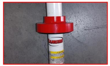
Install shock into to spring. Using the spring compressor, Compress spring and install the factory shock nut. Tighten and torque to 30 ft-lbs.
