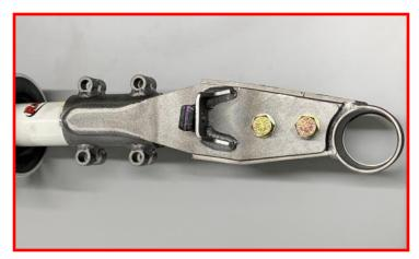
Using the provided M10 x 40mm bolts, washers and locking nuts, Install the strut bolts from bottom up through the strut extension and factory cross pin.
