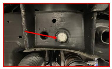
Using the inside edge of the rear control arm/ rear crossmember pocket, measure towards the outside of the vehicle frame 1.625" and make a vertical mark on both sides of the frame. Connect the two lines across the top of the frame rail. Using an appropriate cutting tool, cut through marked line. Sand the cut surface to remove any sharp edges. Paint the cut surface to prevent any corrosion.
