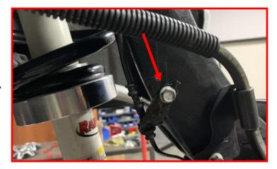
Install brake line bracket to the back of knuckle using the factory mounting hardware.
