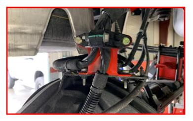
Install the rear wheels and lower vehicle to the ground. Torque the lug nuts to the wheel manufacturer specs, the U-bolts to 110 ft-lbs and all shock hardware to 65 ft-lbs.
