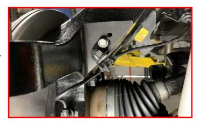
Install ABS sensor harness bracket to the back of knuckle by flipping bracket over and mounting bracket with the factory mounting hardware.
