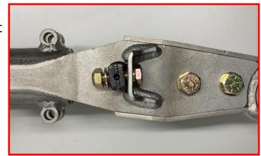
Install the M10 x 50mm bolts, washers and locking nuts from back to front.
