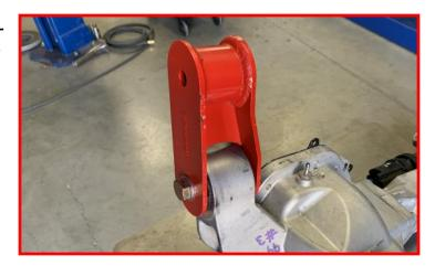
Install differential drop bracket crush sleeve in the factory differential frame mount located on the passenger side. Make sure the crush sleeve is fully inserted prior to installing the differential.
