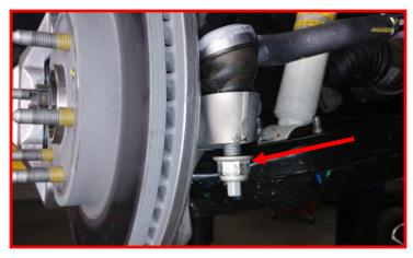
Remove the ABS bracket from the upper control arm. Remove ABS sensor harness from bracket and discard bracket.
