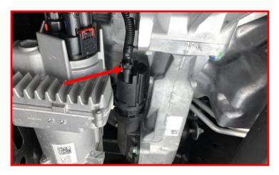
Remove differential vent line from the top of the differential.
