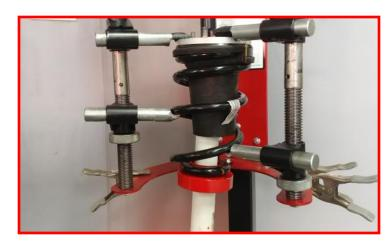
If the strut still has the lower clip nuts attached, remove and discard.
