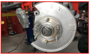
Install the upper ball joint to the knuckle using the provided hardware.
