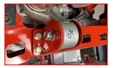
Tighten passenger differential drop bracket hardware.
