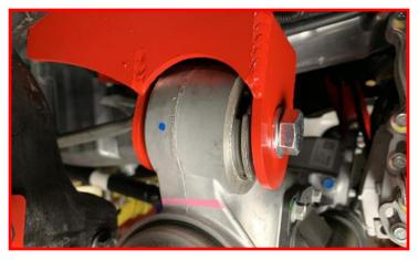
Tighten driver differential drop bracket hardware.
