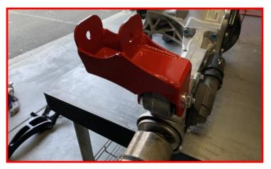
Install driver side differential drop on factory differential mounting point using the supplied M14 x 90mm bolt, washers and nut. Do not tighten at this time.
