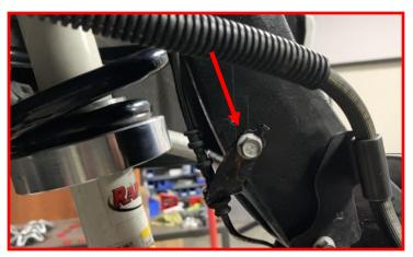
Install brake line bracket to the back of knuckle using the factory mounting hard-ware.
