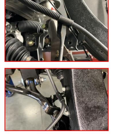
Using a couple wire ties, secure the ABS sensor harness to the brake line.
