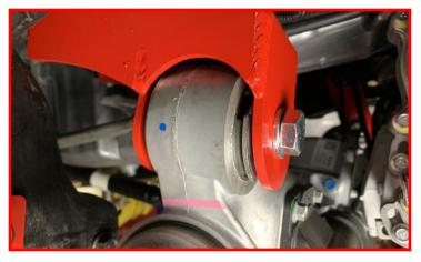
Tighten driver differential drop bracket hardware.
