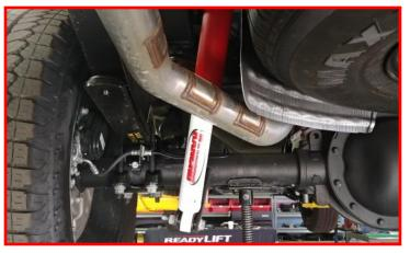
Remove the driver side U-bolts completely and discard. Lower the axle enough to ensure clearance to install lift block making sure that all brake lines and ABS lines do not get over extended.
