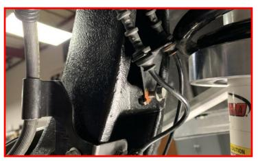
Using a couple wire ties, secure the ABS sensor harness/ brake pad sensor to the brake line.
