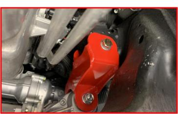
Install passenger differential drop bracket using factory hardware. Do not tighten at this time.
