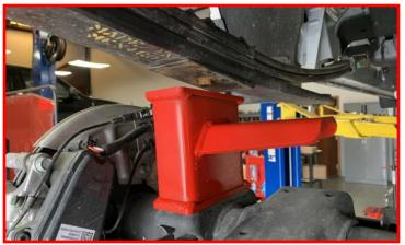
Install the provided U-bolts, and nuts. Snug the U-bolt nuts but do not fully tighten at this time. Repeat steps for other side.
