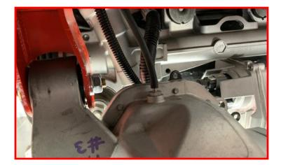
Tighten rear differential drop hardware. Torque M14 hardware to 120 ft-lbs.
