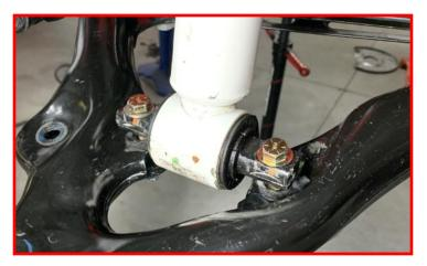
Swing lower control arm up, Install supplied M10 bolts through strut cross pin and lower control arm. Install M10 washers, and nuts on to bolts.
