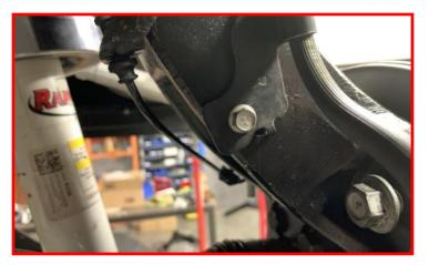
The brake line bracket may need to be moved down the brake line in order to avoid straining the brake line.
