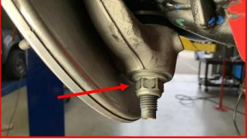
Remove the lower control arm from the frame. Be sure to retain factory alignment cam bolts, cams and nuts.
