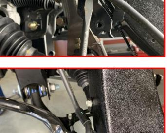
Install ABS sensor harness bracket to the front of knuckle using the factory mounting hardware.
