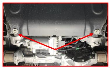
Loosen the top strut nuts but do not remove at this time.
