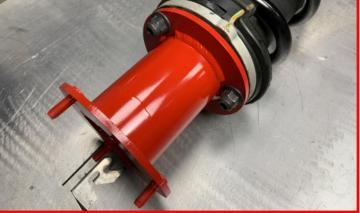
If the strut still has the lower clip nuts attached, remove and discard.
