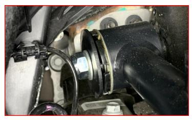
Once upper control arms have been properly torqued, install completed strut assembly. Install with supplied M10 nuts.
