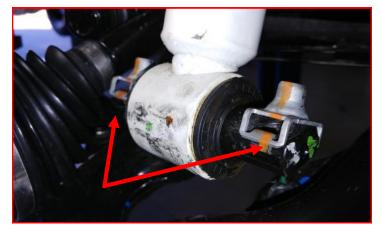
Prior to installation, ensure you have the proper replacement control arm, they are side specific and need to be install on the correct side.
