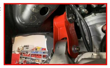
Install rear crossmember using the supplied cam block off plates, M18 bolts, washers, and nuts. Do not tighten at this time.
