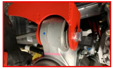
Tighten driver differential drop bracket hardware.
