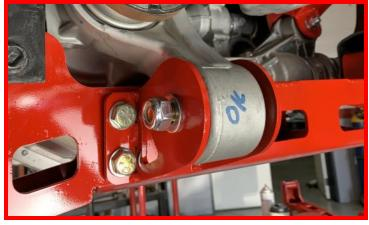
Tighten passenger differential drop bracket hardware.
