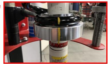
Install front strut spacers using factory nuts.
