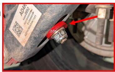
Install shock into extension using supplied M14x80mm bolt. DO NOT TIGHTEN AT THIS TIME.
