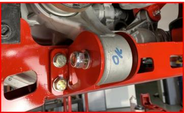
Tighten passenger differential drop bracket hardware.
