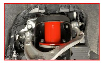
Remove the lower nut clips from the strut and discard.
