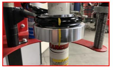
Install front strut spacers using factory nuts.
