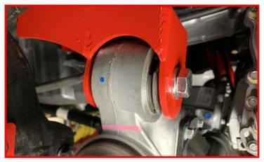
Tighten driver differential drop bracket hardware.
