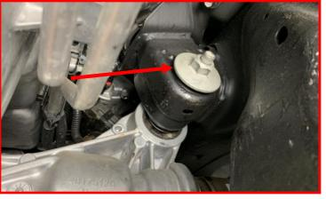
Measure from the pinion seal forward 6" and mark location. Measure from the outside of the fin inward approximately .375" and mark the location. Connect the two marks. Using an appreciate cutting tool cut away the material while following the marked line. Repeat steps for the bottom fin as well.
