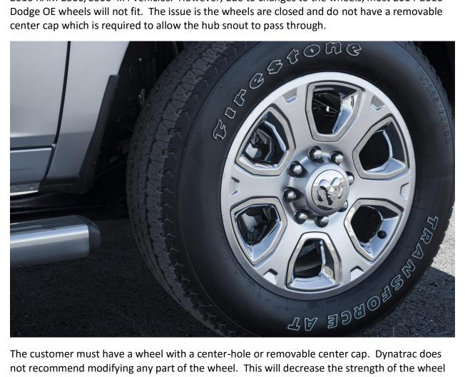
The customer must have a wheel with a center-hole or removable center cap. Dynatrac does not recommend modifying any part of the wheel. This will decrease the strength of the wheel and can lead to catastrophic failure. Most aftermarket wheels will have a removable center cap, but the customer must confirm before ordering. Dynatrac has confirmed the fitment of the following wheels:
