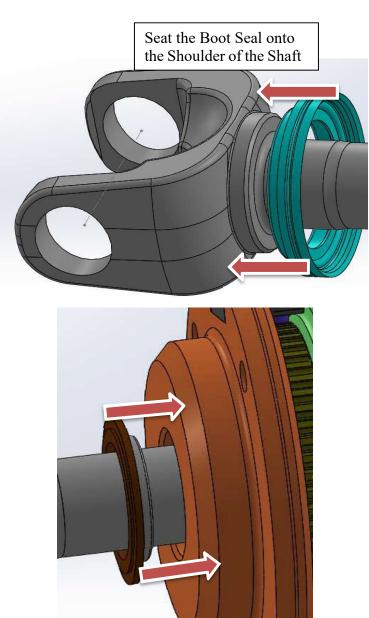
Tap Thrust Washer Into the Back of the Spindle
