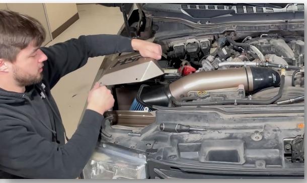
**38.** Tighten clamps on the throttle body, air intake pipe and filter
