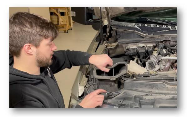
**16.** Disconnect the front half of the scoop from the OEM battery tray by removing the 2x 8mm bolts
