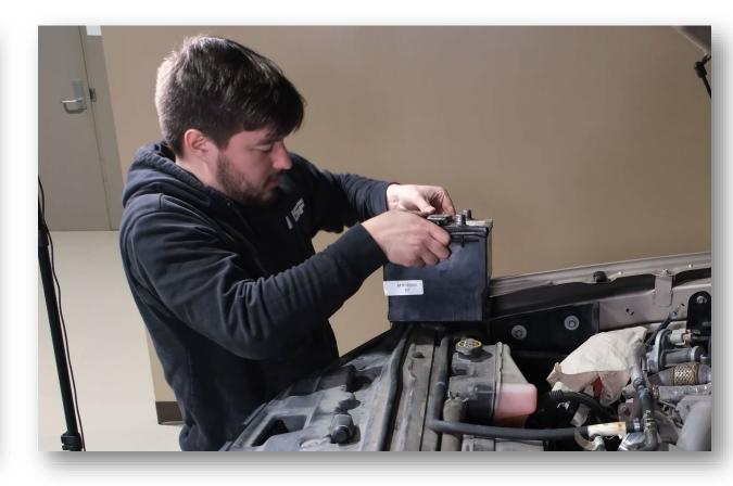
**13.** Use a 13mm socket and extension to remove the 4 battery tray bolts from the truck
