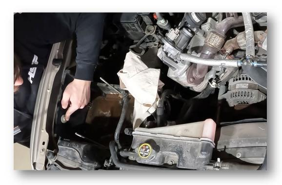
**14.** Disconnect the intake scoop by prying up on the push pin connector with a flathead screwdriver
