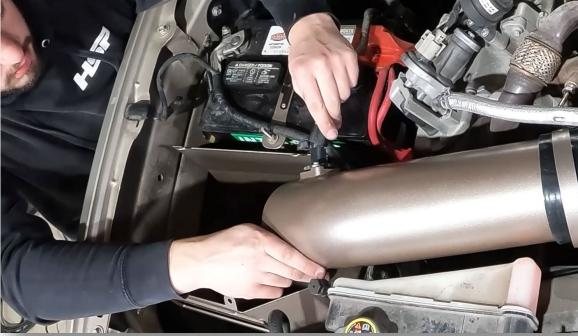
**37.** Put air filter on the intake tube and align filter with hole in box
