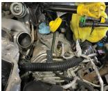
**Note:** This could be an optional step depending on your skill level, or if you are upgrading the hot side pipe also. Locate locking clip on factory intercooler pipe at turbo as shown. Using two screwdrivers or pick tools, release clip by gently prying up under it from turbo side of factory intercooler pipe. Pull boot off turbo. Loosen clamp on intercooler pipe at factory intercooler. Remove factory turbo hot side pipe from vehicle and set aside.
