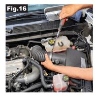
Step 13. Secure the coupler onto the air cleaner lid, and reconnect the MAF sensor to the factory location. (Fig. 16)
