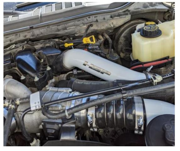
2011-2022 Ford 6.7 Powerstroke Hot Side Charge Air Pipe
