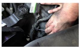
4. Release the clip holding the wires on the ECM cover. Push the wires to the side.
