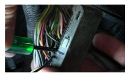
10. Use a sharp tool to poke through the insulation of terminal 71.
