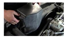
1. Remove the two bolts holding the TCM cover on and lift up the cover.
