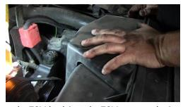
15. Snap the TCM back into the TCM cover and reinstall the cover using the two bolts.
