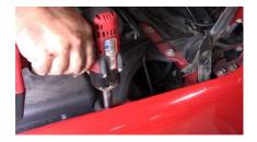
16. Up at the fire wall remove the fender brace.
