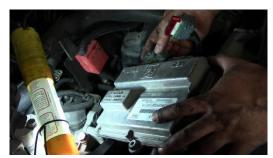
14. Clip the wires back into the ECM cover. Plug the connectors back into the TCM. Note the color of the connectors match the labels on the TCM.
