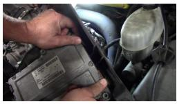
2. Release the tabs holding the TCM into the cover.
