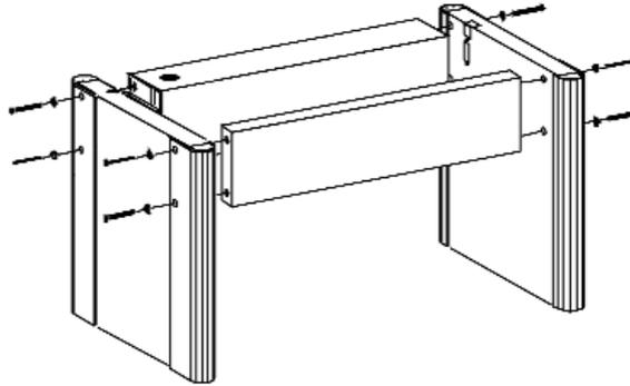
**3.2.6** Tighten all eight screws securely with a slotted screwdriver.
