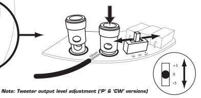
On some Q Install models the tweeter output level can be increased or decreased using the 3 position switch located at the rear of the product. It is recommended to leave the switch in the 'O' position for the initial sound check.
