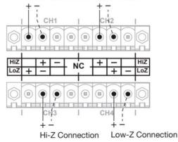
Ch1: Low-Z connection Ch2: Hi-Z connection Ch3: Hi-Z connection Ch4: Low-Z connection
