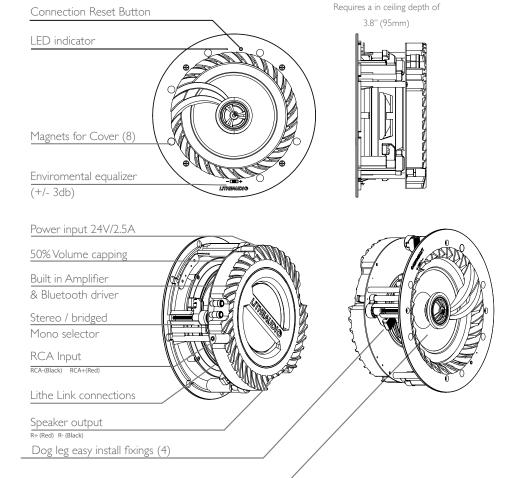
In built over voltage, under voltage, over temperature, and short circuit protection, if there is an electrical fault, the power supply to the amplifier will cut off automatically and restart when the speaker has stabilised.
