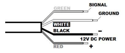
The internal amplifier can be operated from any 12Vdc power supply capable of delivering up to 2A current.
