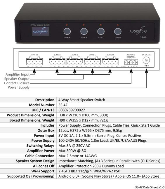
3S-4Z Data Sheet v1-0 © Efficient Technology Ltd
