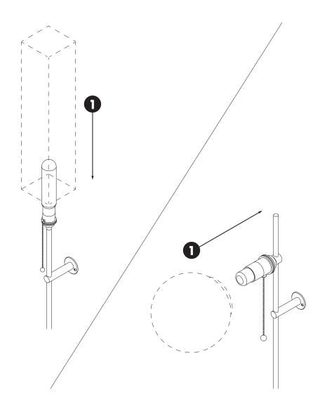
1. Install lamp body onto wall with provided hardware.
