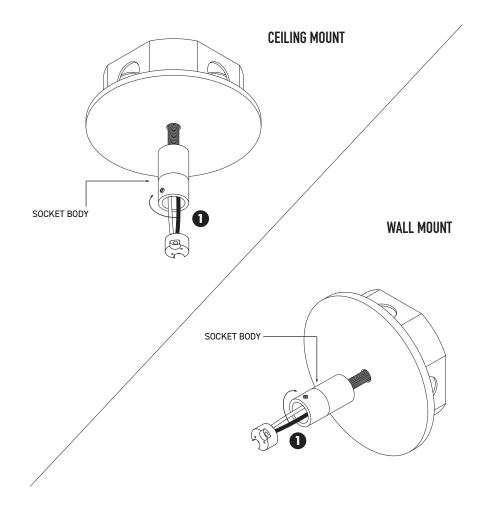
1. Align backplate and fasten socket body to crossbar
