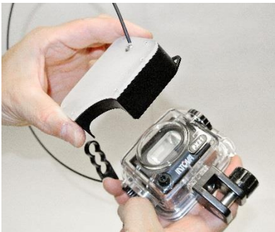
4. Attach diffuser holder to PX-21
