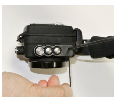
8. Allow cable to "relax" any twist and very carefully tighten hex nut.
