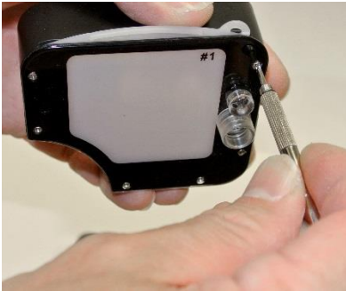
1. Remove front plate from diffuser holder
