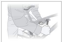
**8.** Once the ring is threaded off the shock, the forward end of the shock will extend forward to reveal an o-ring, a round metal plate and the spacer.
