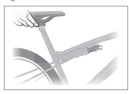
**16.** Use the BSA30 tool to turn the lock ring onto the strut.
