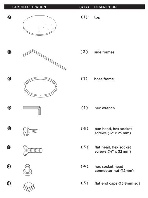
ATTENTION: USE THE CARTON AS A WORKING SURFACE TO PREVENT TABLE-TOP DAMAGE DURING ASSEMBLY.
