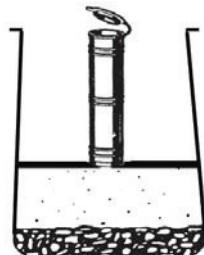
Pour about 6" of concrete into hole (or until it comes to the bottom of the ground sleeve).
