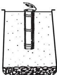
Position ground sleeve as shown and pour concrete around the outside until flush with the top of the ground sleeve (or 1-1/2" below top if in lawn). This will allow filling top layer with soil and planting.
