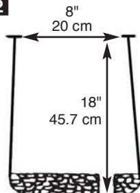
Dig hole 8" to 12" in diameter and 16-18" deep. Taper hole larger at bottom. Fill bottom of hole with small rocks approximately 3" deep.
