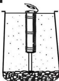
Immediately run a small tube or stick down the center of the sleeve through the concrete until it reaches the crushed rock base. Remove tube or stick. This will allow any water to drain.
