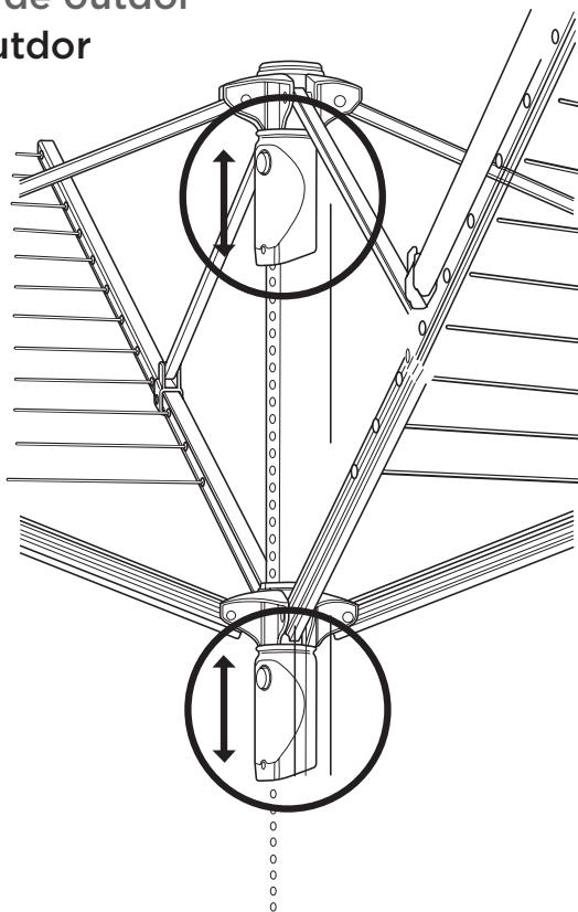
**HANDLE OPERATION:** Push in release button on lower handle grip. Slide handle up pole to desired height. Release button and lock into a hole on the center pole. To tighten lines, push in release button on the top handle grip and slide down center pole.
