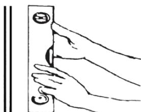
Insert pole into ground sleeve and use a level to align the pole vertically. Carefully remove pole, without moving the ground sleeve.
