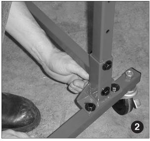
Remove right side "B" Series leg support tube. Transfer wheels to "C" Series leg support tube. Fasten "C" Series leg support tube to frame. Repeat for left side.
