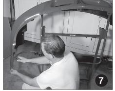
Mounting Bumper Cover. With the cradle support in a downward position, center the bumper cover on the foam pad. Adjust crosstube to proper length of bumper ends. Tighten knobs. Adjust support arms to proper width of bumper and tighten knobs.
