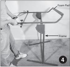
Using four 1½" bolts with washer and nuts, mount cradle tube assembly to frame (as shown).
