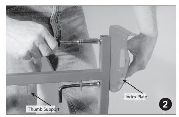
**Install Index Plate.** Use a 7/16 socket to slide push clip onto the index plate rivet.
