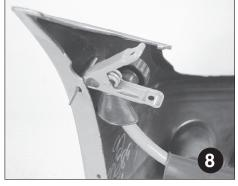
Clamps and/or Pins. Use pins to secure bumpers when possible to assure full paint coverage. Maximum weight 11 kg..
