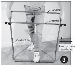
Cradle Assembly. Slide handrail into crosstube. Insert two plastic knobs, then tighten. Then slide handrail into cradle tube only to first hole (see arrows in photo).
