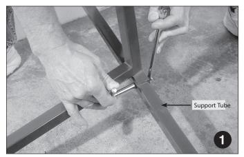
**Install Support Tubes.** Install plastic end caps and bolt on the foot pads using  $\frac{1}{2}$ " flat washer with nut. Then, using four  $\frac{1}{2}$ " bolts with washer and nuts, mount support tube to frame. Then, install wheels.
