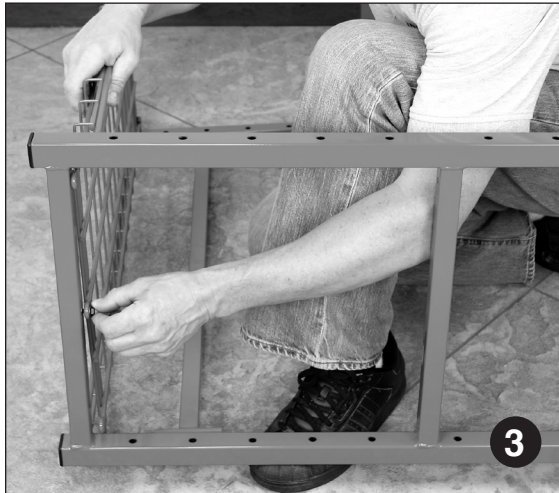
Lay Material Cart flat with Crosstube on floor. Install top shelf using only 1/4" x 3/4" bolts and washers. (Note: smaller wire on top side of shelf.)
