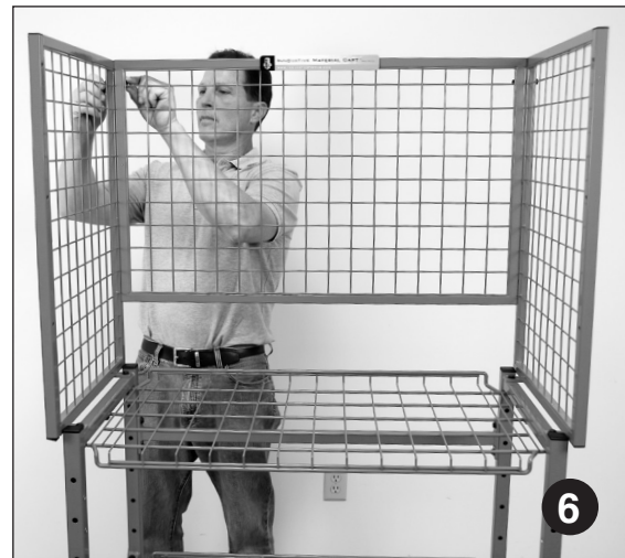
Install Upper Back Frame P/N 730-014 using 1/4" x 2" bolts with corresponding nuts/washers. Tighten all hardware.
