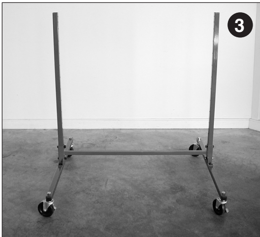
3 Slide longer side rail tubes (P/N 290-005) into lower base support, insert bolts. Note: do not tighten bolts until frame is completed.
