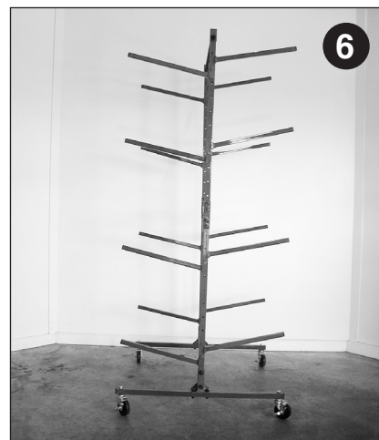
6 Put support arms in desired positions. Note: the four longer support arms are normally in the topmost positions.
