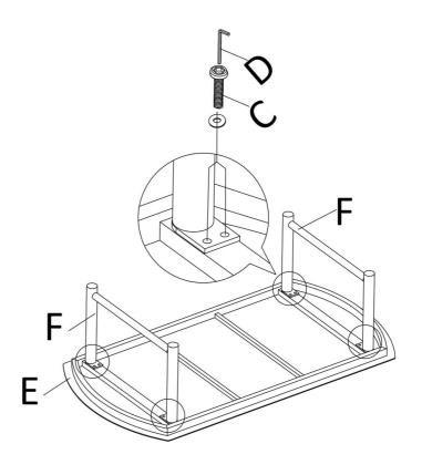
STEP 2 Ensure the screws are tightened and the assembly is complete
