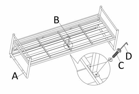
STEP 2 Ensure the screws are tightened
