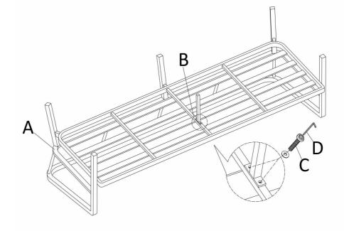
STEP 2 Ensure the screws are tighten
