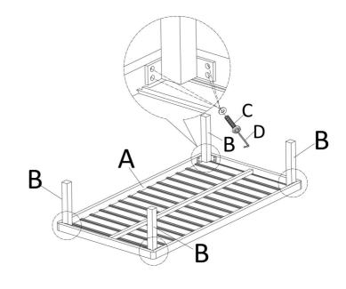
STEP 2 Ensure the screws are tightened and the assembly is complete
