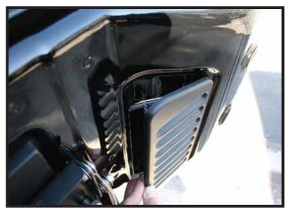
3. Place the UFO and the 1/4" flat head bolt through the outside of the tailgate and secure them from the inside using the fender washer and the nylock nut. Take extra caution as to not drop the hardware inside the tailgate! Tighten only until snug using a 5/32" hex L-key and a 7/16" open end wrench.
