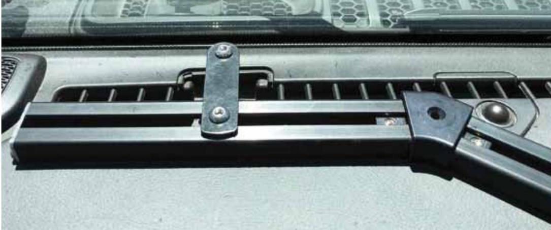
6. You can loosen and adjust the edock pieces to make slight adjustments to the contour.
