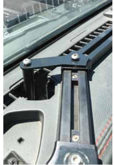
4. The driver side bracket connects to the track with a drop in anchor. Install the anchor into the track at an angle and then use small tool to rotate it flat. Position the anchor directly in front of the standoff.
