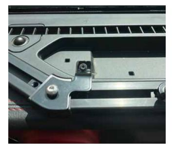
2. There is a bolt below each of the dash caps that were removed on page 2. Remove the Driver side bolt and carefully thread the standoff into the hole. Remove the passenger side bolt and install the spacer first and then thread in the standoff. It may be helpful to use a little bit of tape to secure the spacer to the bottom of the standoff to get everything aligned. You can slip a washer in between bolt and the standoff to help tighten it down.
