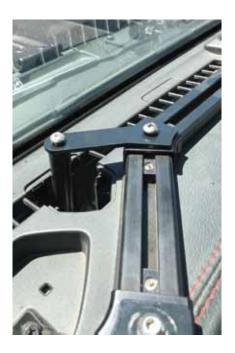
4. The driver side bracket connects to the track with a drop in anchor. Install the anchor into the track at an angle and then use small tool to rotate it flat. Position the anchor directly in front of the standoff.
