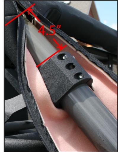
4. Pull the roll bar padding back around the clamps (Leave unzipped). The velcro opening in the padding should align with the mounting face of the clamps. A second person or something to support the basket is helpful for the following step. Lift the basket into place and fasten both brackets to the clamps using eight 1/4-20 x 1/2" Flange head bolts. Keep the hardware loose at this time.
