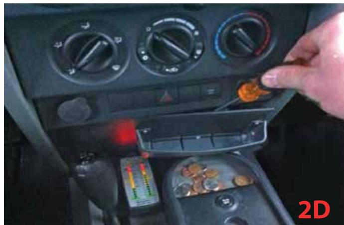
E. Remove the four screws (using a 7mm socket) to release the large radio and climate control trim piece. There are two screws on the top and two on the bottom. After all four screws are removed, GENTLY pry the lower corner of the trim piece working side to side and bottom to top until all of the snaps have released. Do not disconnect any of the wires connected to the trim piece. Let the trim piece rest against the shifter.
