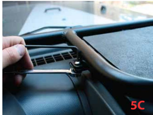
C. Place a socket head screw through the top of the Hoop Tabs and down through the Hoop Support Legs and secure with a nylock nut using a 5/32" Hex Key and a 7/16" open end wrench. Repeat for both sides of the hoop.
