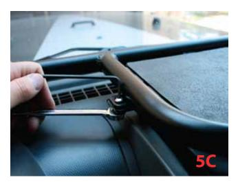
C. Place a socket head screw through the top of the Hoop Tabs and down through the Hoop Support Legs and secure with a nylock nut using a 5/32" Hex Key and a 7/16" open end wrench. Repeat for both sides of the hoop.
