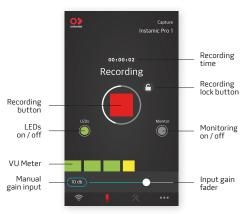
**RECORD** Tap on the Recording button to start capturing. If auto-gain is selected, Instamic will starts recording after measuring the input gain on the first 8 secs.
