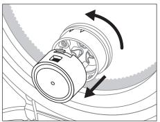
To replace, align the square opening in between the 2 arrows indicated on the Steam Vent and turn clockwise until it clicks.
