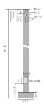
The LED Straight Square Steel poles are built from high strength steel tube and are available side drilled for arm mounted area lighting luminaires or with tenon mounts of flood and post top luminaires. Typical area lighting applications include retail centers, industrial parks, schools and universities, public transit and airports, office buildings and medical facilities. Mounting heights of 10 to 30 feet can be used based on selected luminaires, application.
