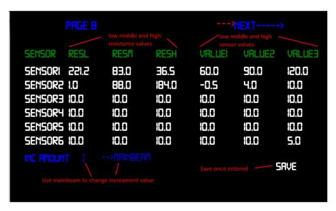
Enter the calibration data for your oil temp and pressure sensors Use Celsius for temp and Bar for pressure
