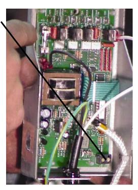
2. Insert one of the thermostat wires into each of the terminals on the bottom of the J18 thermostat connection block and tighten the screws on the front of the thermostat terminal. The thermostat wires should be securely held in place by these screws (remember that the thermostat is not polarity specific, so it will not matter which wire goes into either terminal).
