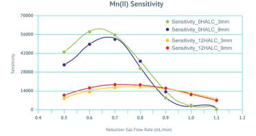
Figure 4 highlights the effect of nebulizer depth on Mn (I) and Mn (II) sensitivities as a function of nebulizer gas flow rate for two different height above the load coil (HALC) positions and two different nebulizer depths (3mm: closer to the aerosol impact zone and 9mm: away from the aerosol impact zone).
