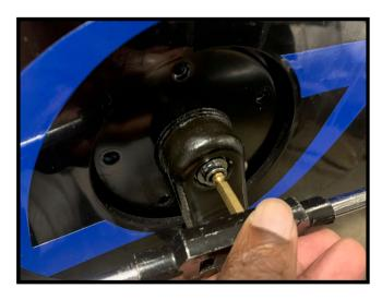
Once the hole is drilled into the center of the bolt, use a easy out/screw extractor to remove the crank bolt.
