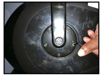
Apply grease to the bottom bracket splines before installing the new right crank. Install the new right crank 180 degrees (opposite) from the left crank. Tighten the middle crank bolt onto the bike. Ensure to insert the 8mm Allen key fully into the bolt to prevent damaging the new crank bolt. Next line up the (5) bolts on the outer ring with the pulley,
