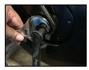
Attach the nut from the crank puller into the crank arm. Then tighten the nut with a adjustable wrench.
