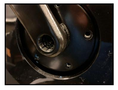
Now that the bolt is removed, you can now remove the crank using a crank puller (CCP-44).
