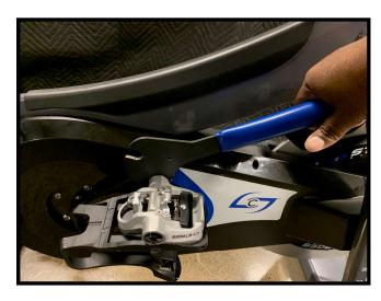
Apply a dab of blue Loctite onto the treads of the pedal, then reattach the right pedal and screw it in as far as you can by hand then with a 15mm pedal wrench completely tighten.
