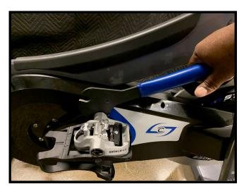
Apply a dab of blue Loctite onto the treads of the pedal, then reattach the right pedal and screw it in as far as you can by hand then with a 15mm pedal wrench, then completely tighten.
