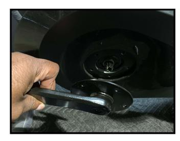
Turn the crank puller clockwise until the crank pulls off the bottom bracket.
