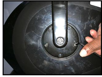
Apply grease to the bottom bracket splines before installing the new right crank. Install the new right crank 180 degrees (opposite) from the left crank. Tighten the middle crank bolt onto the bike. Ensure to insert the 8mm Allen key fully into the bolt to prevent damaging the new crank bolt. Next line up the (5) bolts on the outer ring with the pulley,
