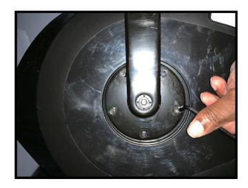
Remove four of the five bolts on the outer ring of the right crank/pulley with a 5mm Allen key, then only loosen the last bolt.
