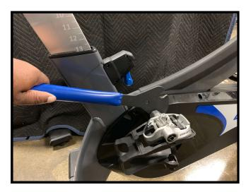
Turn resistance knob all the way clockwise or push down resistance knob to apply the brake on the bike, then remove the pedal from the right crank arm using a 15mm pedal wrench.
