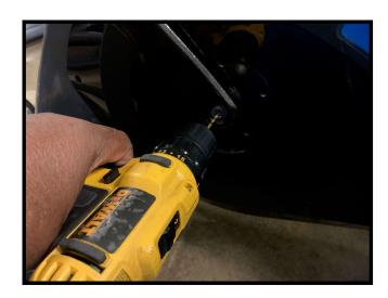
With the punch made, begin drilling in the punch straight in the middle of the bolt.
