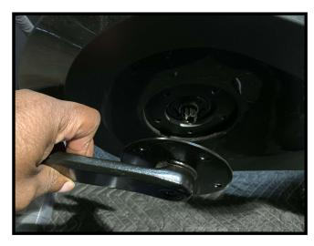
Use a 8mm Allen key to extract the right crank arm off the bottom bracket and then remove the last bolt on the outer ring of the pulley to remove the right crank arm. Ensure that the Allen key is fully inserted into the bolt, allowing you an opportunity to release the bolt from the crank.
