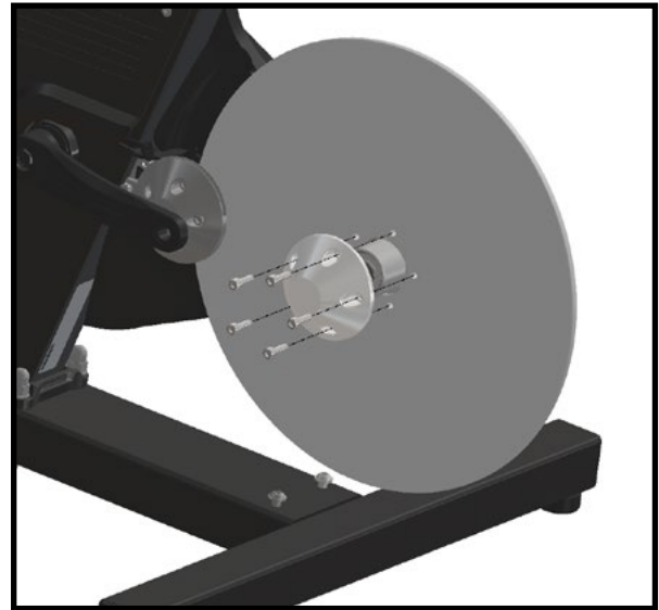
Figure 4. Flywheel and Hubcap Installation
